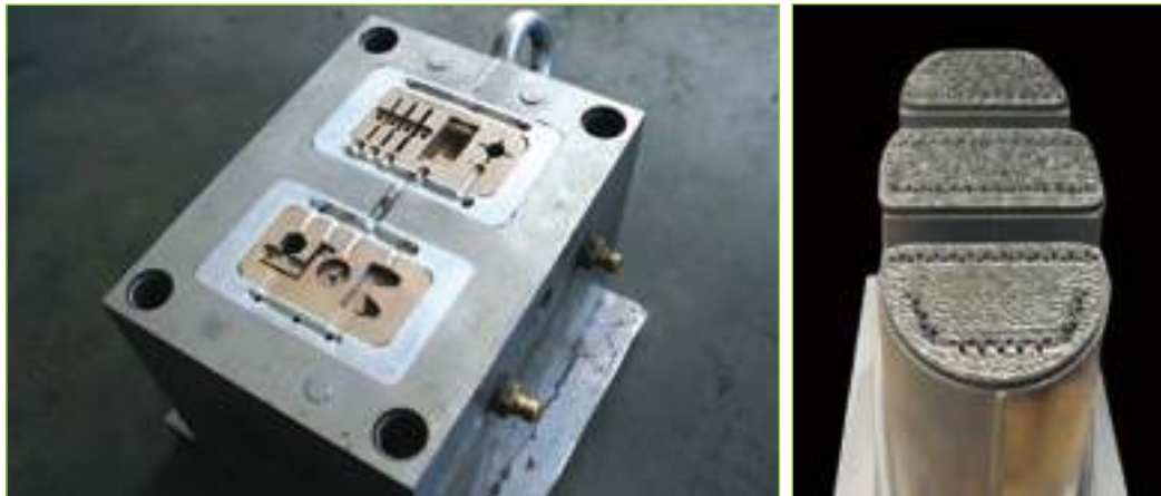
Examples of tooling inserts and conformal channels produced using AM (Source: Product Development Technology Station, CUT and Stellenbosch University)
