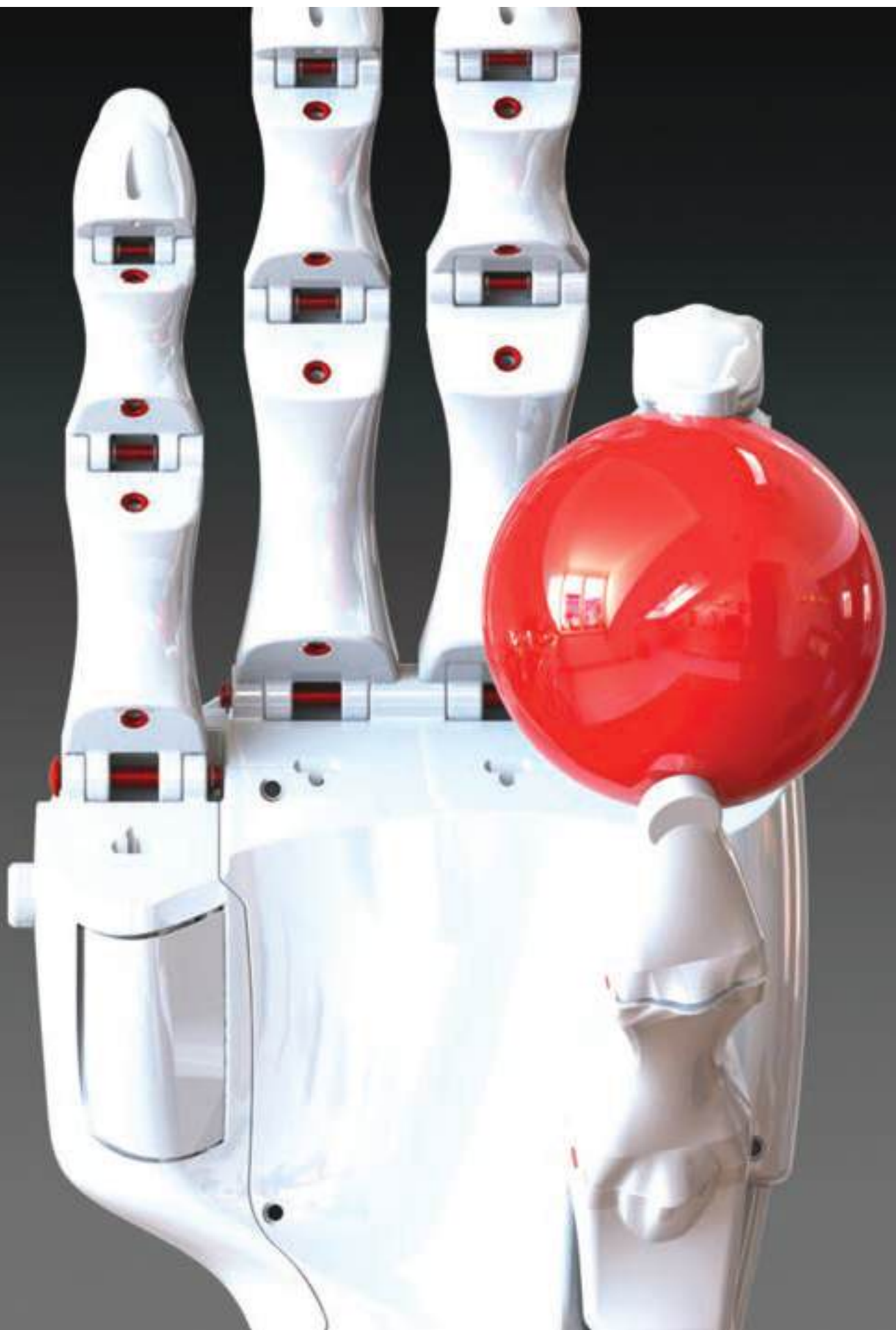
Anthropomorphic prosthetic hand (Source: George Vicatos and Severin Tenim (UCT))
