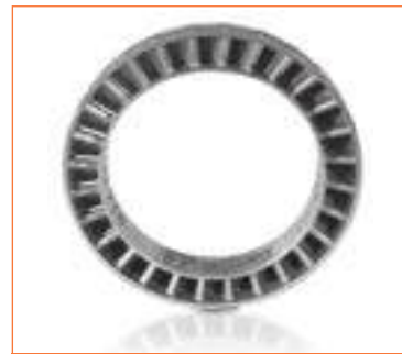
Stator ring in IN718 (Source: Morris)
