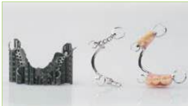
Partial denture manufacturing stages (Source: EOS)
