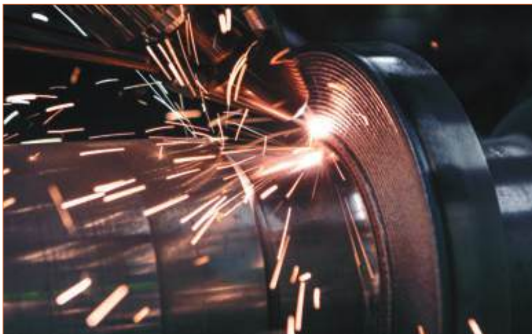
Laser Metal Deposition technology for refurbishment of high value components (Source: CSIR National Laser Centre)
