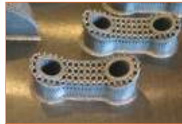
Osseointegration Ti implants (Source: ATTRI Orthopaedics)
